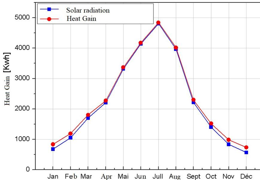
Figure.5. Heat Gain
